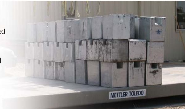
NTEP testing of a scale's CLC using a large test pattern
