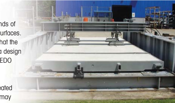
Module being accurately loaded at the rated capacity
